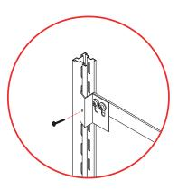
The metal bar can be screwed securely to the vertical uprights using the screws provided in the package. To do it take the screws, place them in the holes of the hooks of the metal bar and screw them in with a drill (the screws will independently drill into the uprights).
